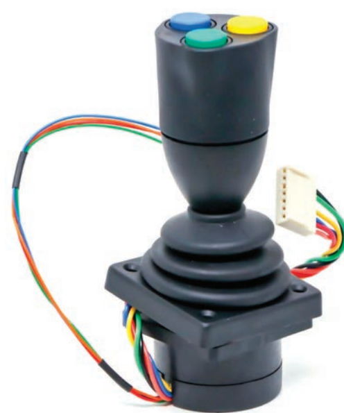
APEM Seria 3000 – MPN 3140SBB6475 Joystick, 2 – Axe, Analogic (Efect Hall) Ieșire tensiune: \pm 10\% \times V la \pm 50\% \times V
